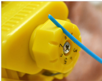
Built-in sizing channels determine proper setting for buffer tubes.
